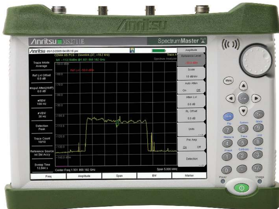
Spectrum Master TM MS2711E Spectrum Analyzer featuring 8.4 inch Daylight Viewable Touchscreen Compact Size: 273 mm x 199 mm x 91 mm (10.7 in x 7.8 in x 3.6 in), Lightweight: 3.45 kg (7.6 lb)
